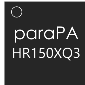
5 mm × 5 mm QFN package
